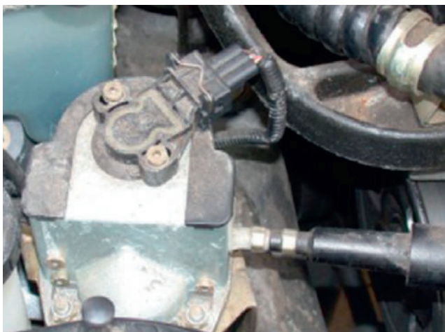
Figure 3.110 Throttle motor connected to cable
